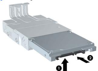
Figure 7-23 Sliding the Hard Drive into the Carrier
